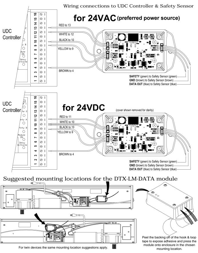
Ensure that wires will reach the UDC controller without binding before mounting the DTX-LM-DATA module. See above. Note: The DTX-LM-DATA module will be functional in any position or rotation.
