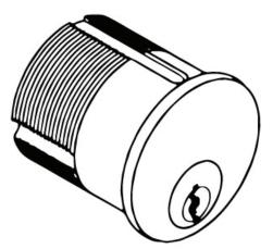
Tailpiece is typically referred to as a cam which is parallel with the back of the cylinder, rotating when the key is turned
