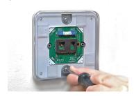
4. Adjust range and delay before activation by turning potentiometer using Philips screwdriver.
