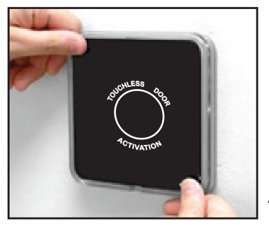
6. Replace faceplate and test unit to ensure proper operation.
