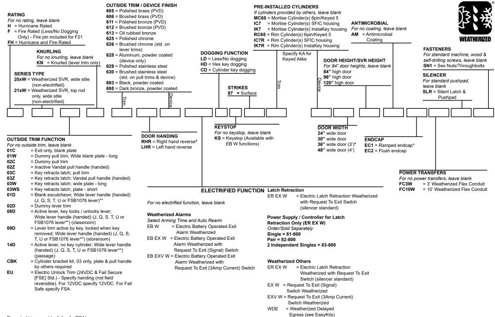
Fire-rated trims must be fail safe (FSA)
