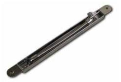
**PT-5** - Power Transfer loops provide a means of running wires from the frame to doors equipped with electric locks and exit devices. The PT-5 is a heavy-duty power transfer device, concealed mortise mount, UL listed miscellaneous fire door accessory. It is UL 10C positive pressure compliant and UBC 7-2 Fire Test for Door Assemblies compliant.
