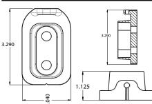
The sill or bottom fitting has a small footprint and, once installed, bottom fasteners are hidden by the mullion tube.
