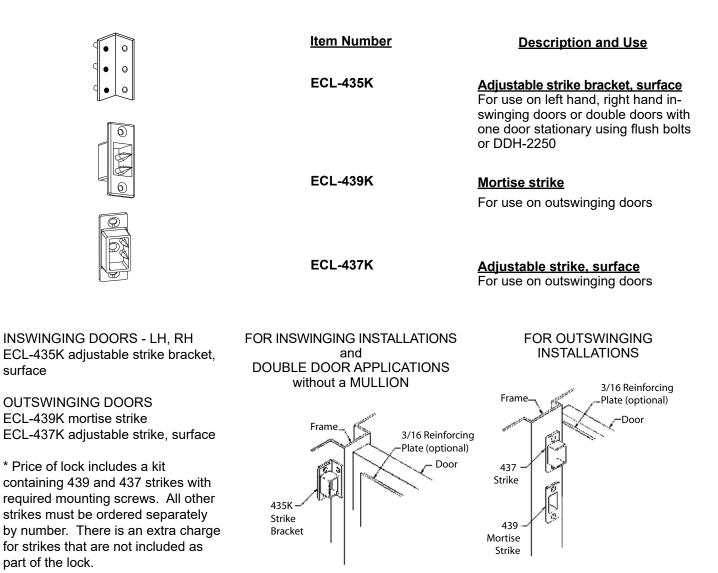
All bracket-mounted strikes include unique adjustable feature for proper installation alignment. All strikes supplied with wood and sheet metal mounting screws.
