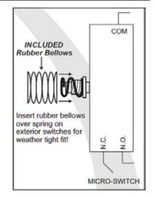
• UL Listed Momentary Switch, SPDT, 15 Amp @ 125V AC  Rubber "Bellows" increases weather protection (included)
