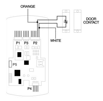
Figure 13: Wiring the Door Contact
