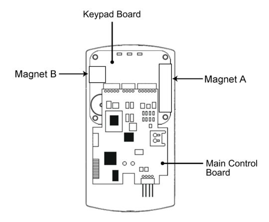
**Figure 5: Tamper Switch Locations**
