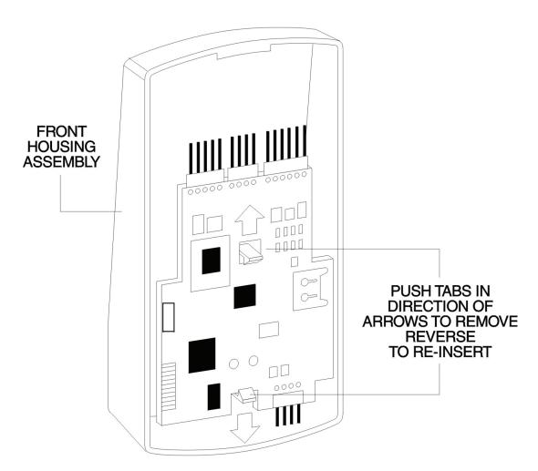
Figure 6: Removing/Inserting Printed Circuit Board
