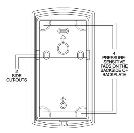
Figure 3: Performing a Glass Mounted Installation
