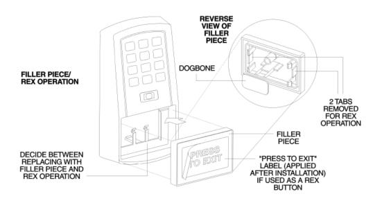
Figure 4: Performing a Secure Installation
