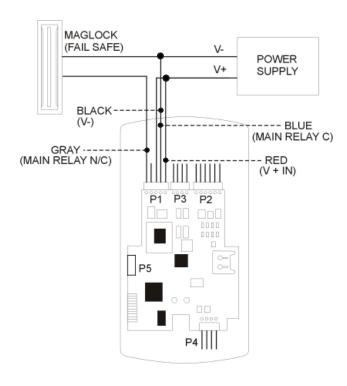
Figure 8: Wiring a Maglock - Fail Safe
