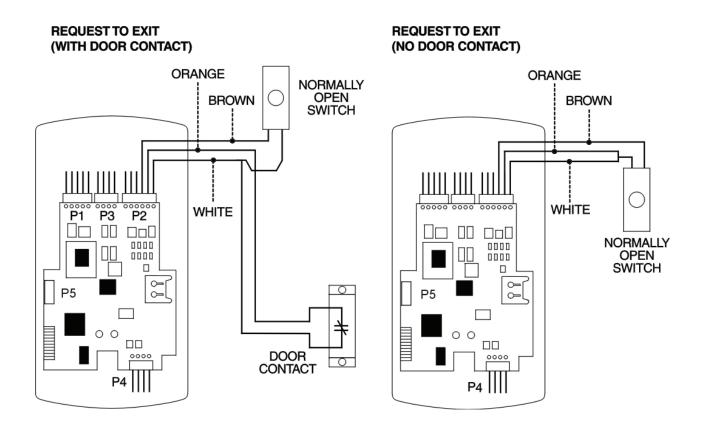
Figure 14: Wiring an External REX Switch
