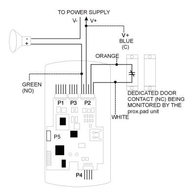
Figure 12: Wiring the Aux Relay For Propped Door
