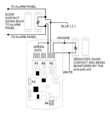
Figure 10: Wiring the Aux Relay for Alarm Shunt
