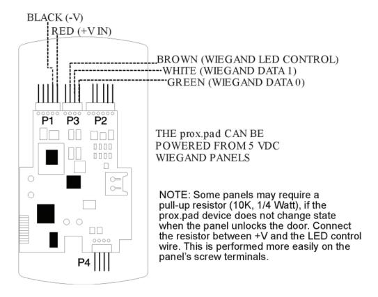
Figure 15: Connecting the prox.pad to a Wiegand Panel
