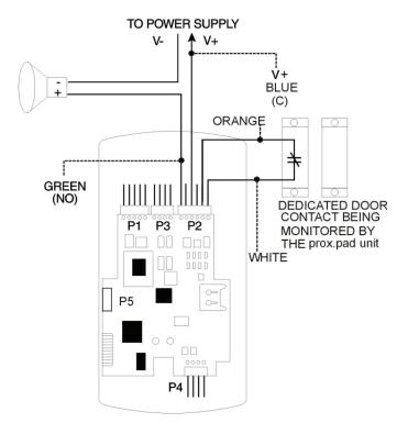
Figure 11: Wiring the Aux Relay for Forced Door
