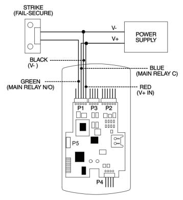
Figure 9: Wiring an Electric Strike - Fail Secure
