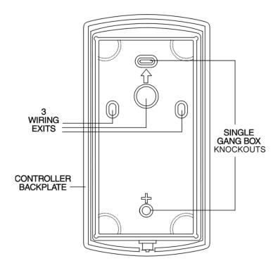
Figure 2: Performing a Wall Mounting Installation
