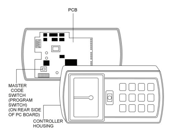
Figure 7: Program Button Location on Main Circuit Board
