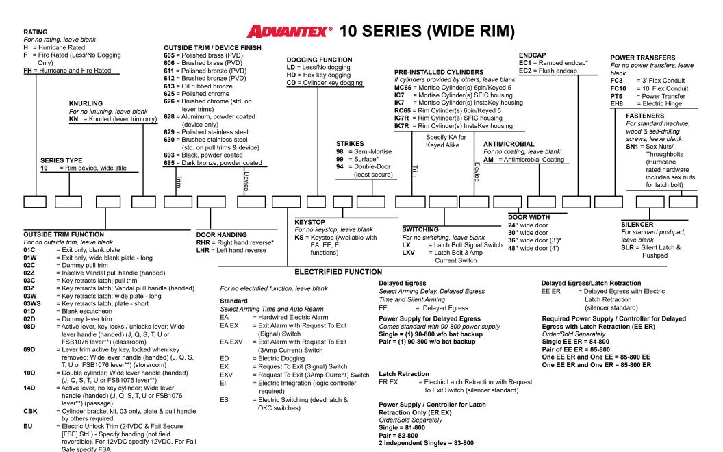
Fire-rated trims must be fail safe (FSA)
