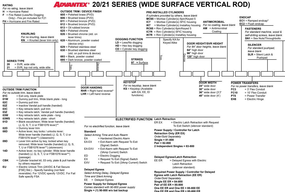
Fire-rated trims must be fail safe (FSA)
