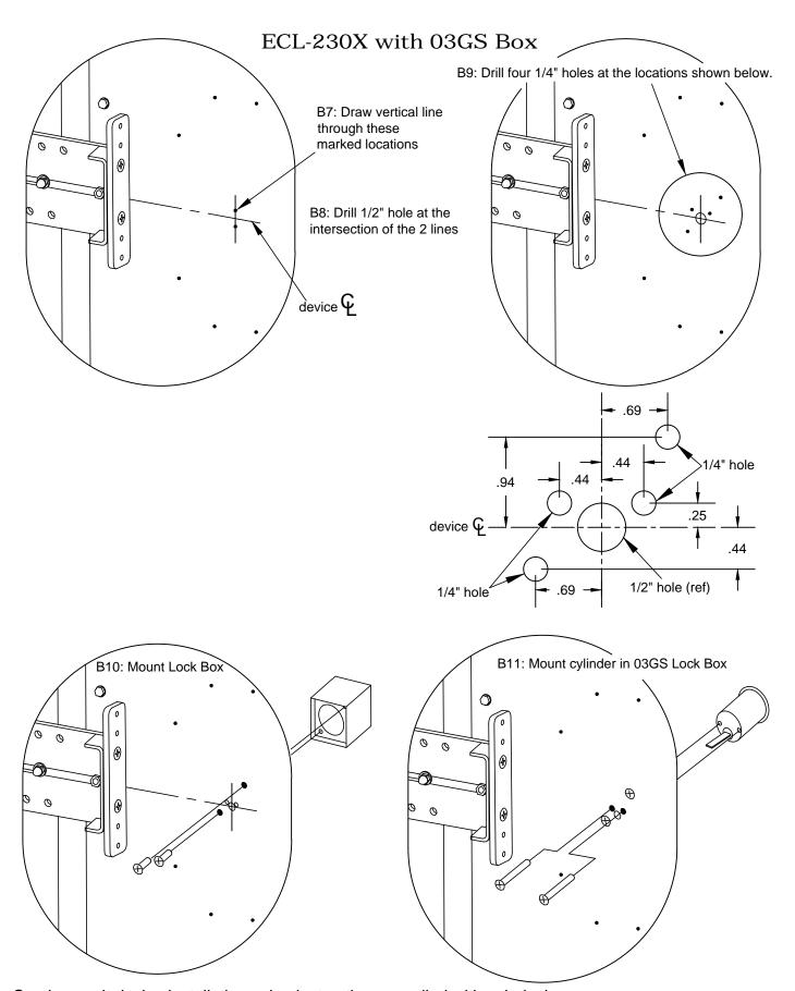
Continue exit device installation using instructions supplied with exit device.
