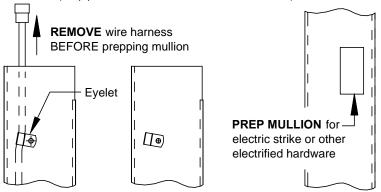
STEP 4: Re-Install Wire Harness & Install Electric Strike or other Electrified Hardware (per Mfg's instructions)
