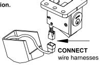
**NOTE:** Connectors are keyed and will only assemble one way
