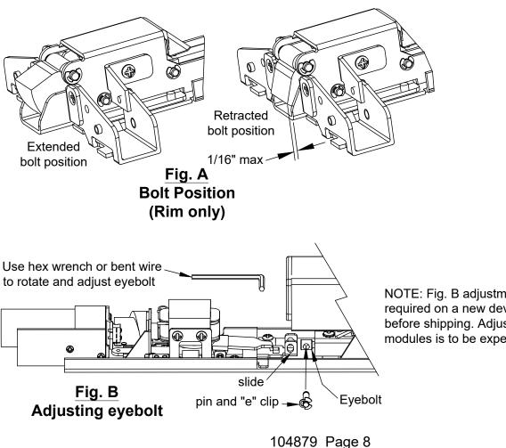
NOTE: Fig. B adjustment should not be required on a new device as they are tested before shipping. Adjustments on replacement modules is to be expected.
