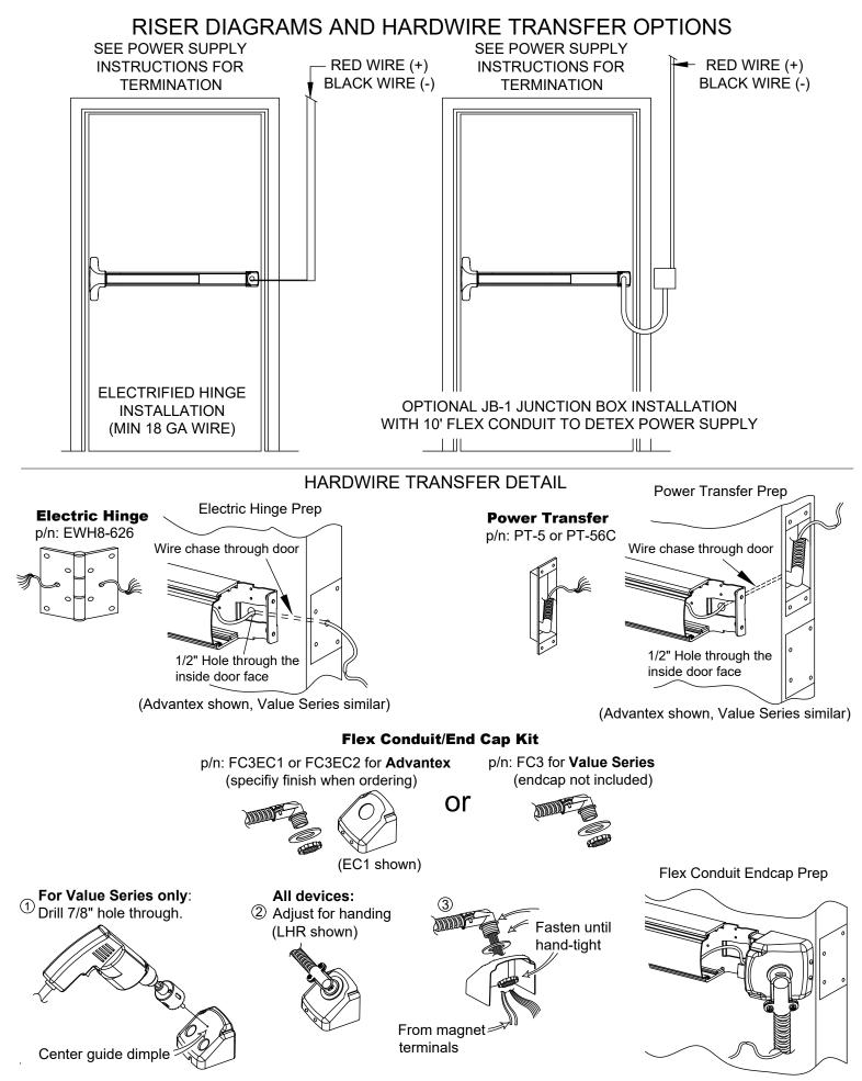
Note: For high traffic areas an electric through-wire hinge or power transfer is recommended.
