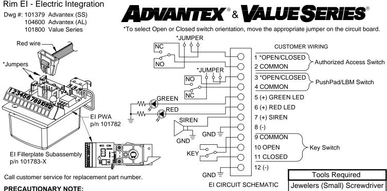
Be careful when installing filler plate assembly not to damage ribbon cable.
