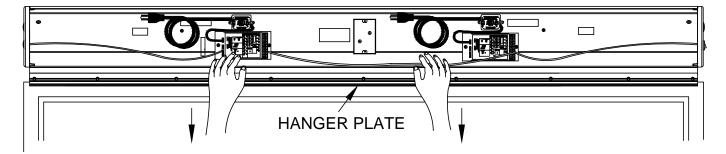
Lift the operator and lower onto the webs of the hanger plate bracket. Be sure both top and bottom are engaged.
