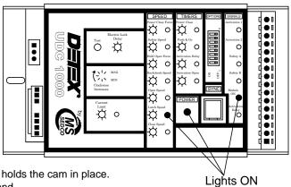
**With door closed:** Using a 1/8th inch Allen wrench, gently loosen the screw that holds the cam in place. Rotate cam in the closing rotation direction until the **Close Speed** light turns off and the **Latch Speed** light turns on. Hold the cam in place while gently retightening the holding screw.
