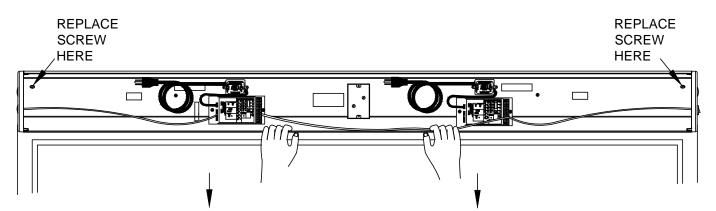
Once they are seated, pull down until unit is completely flush and screws can be replaced in top corners.
