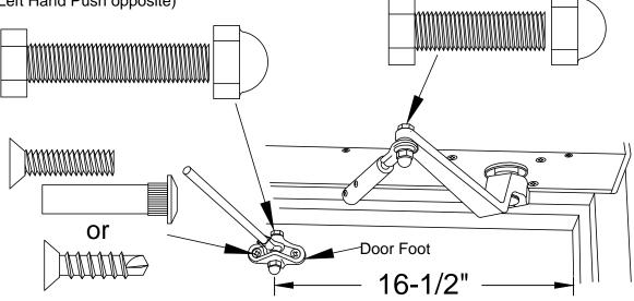
Turn the 3-way toggle switch to the OFF position and close the door. The center of the door foot should be located 16-1/2" from the hinge side of the door frame stop and should be level when the rod is inserted in the sleeve attached to the arm.
