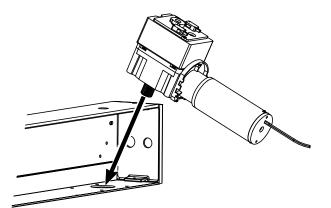
With ASSEMBLY perpendicular to enclosure, insert splined shaft into shaft hole
