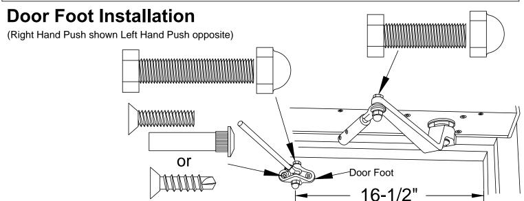
Turn the 3-way toggle switch to the OFF position and close the door. The center of the door foot should be located 16-1/2" from the hinge side of the door frame stop and should be level when the rod is inserted in the sleeve attached to the arm.
