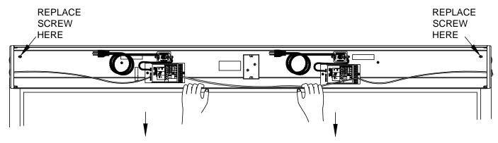
Once they are seated, pull down until unit is completely flush and screws can be replaced in top corners.
