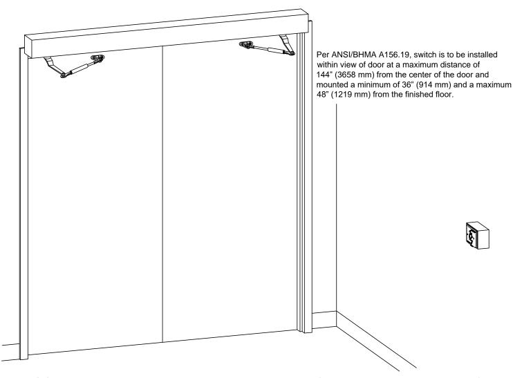
Per ANSI/BHMA A156.19, switch is to be installed within view of door at a maximum distance of 144" (3658 mm) from the center of the door and mounted a minimum of 36" (914 mm) and a maximum 48" (1219 mm) from the finished floor.
