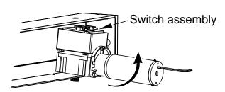
Rotate ASSEMBLY to an almost horizontal position being careful not to let switch assembly hit enclosure
