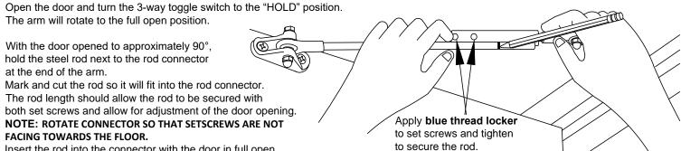
Insert the rod into the connector with the door in full open position and adjust until the desired opening is achieved. Apply **blue thread locker** to set screws and tighten to secure the rod.
