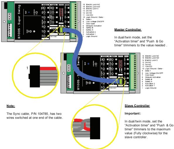
Sensor power can be supplied by both controls for a total of 600mA.
