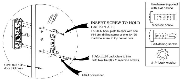
STEP 4: Install Device and Bracket Assembly (LHR Rim installation shown) NOTE: Rim cylinder NOT supplied with trim, but can be ordered separately.
