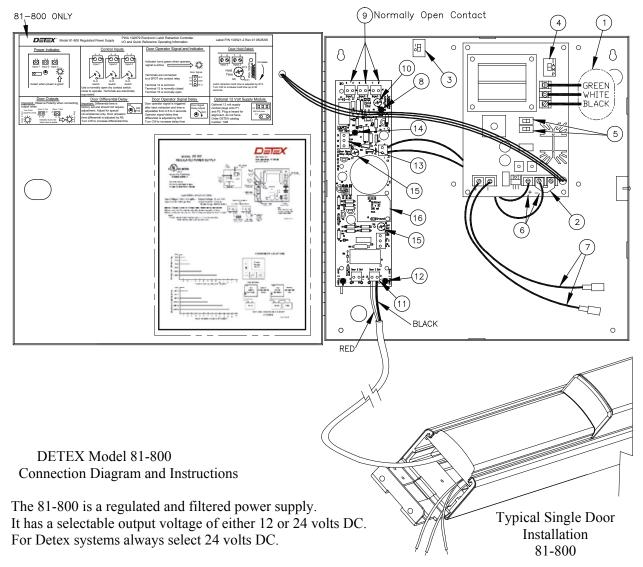
Refer to the drawing of the power supply/controller for connections and adjustments. All connections and adjustment must be made with the power supply de-energized **AND** main power switch (item 3) in the OFF position.
