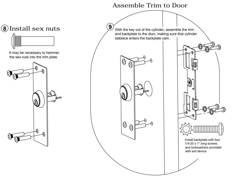
Key should turn freely in both directions when fully assembled to door.
