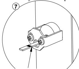
Remove trim assembly from door and cut the tailpiece just inside of the mark. Caution: Tailpiece must not extend past the cam.
