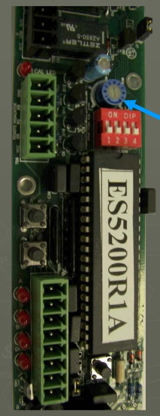
Adjustable Optical Beam Sensitivity
