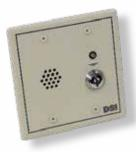
The ES4300A series, used as a stand-alone device or tied to any access control system, provides security for emergency exits. This device activates a local audible alarm and a remote alarm contact when an exit violation occurs. Once triggered, the ES4300 remains in alarm until reset by the auto reset feature, the integral key switch or remotely through a dry contact. The ES4300A is now available with an optional tamper switch.
